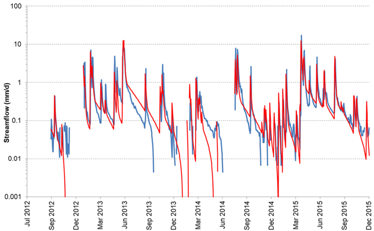
Chart 35 Recorded and Modelled Streamflow Hydrographs for Calibration Period – GS 300077 Honeysuckle Creek
