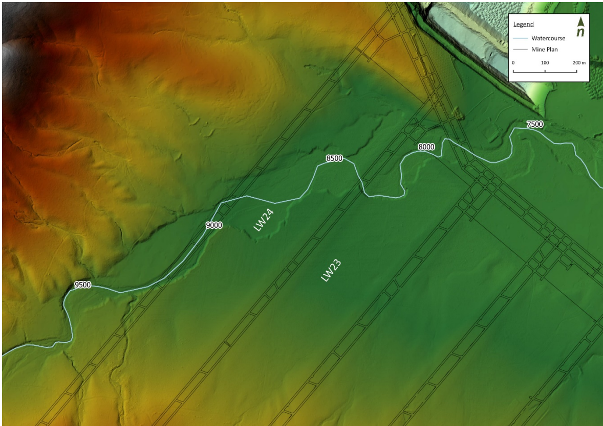
Figure 3-8. Hillshade showing predicted post subsidence surface over LW23 and LW24. Note the extents of macro channel and orientation of the channel in relation to the LW23 and LW24 panel alignment
