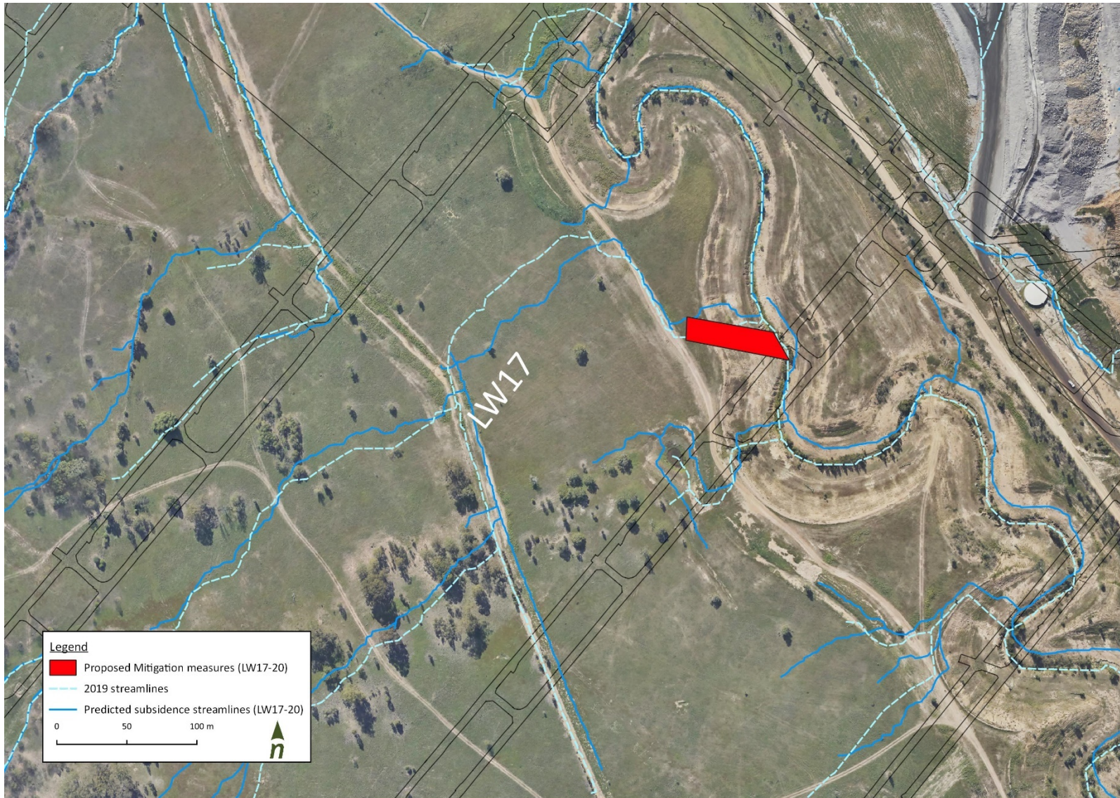
• Figure 4-3. Previous predicted streamlines post LW17 subsidence, including proposed batter chute location, compared to 2019 streamlines
