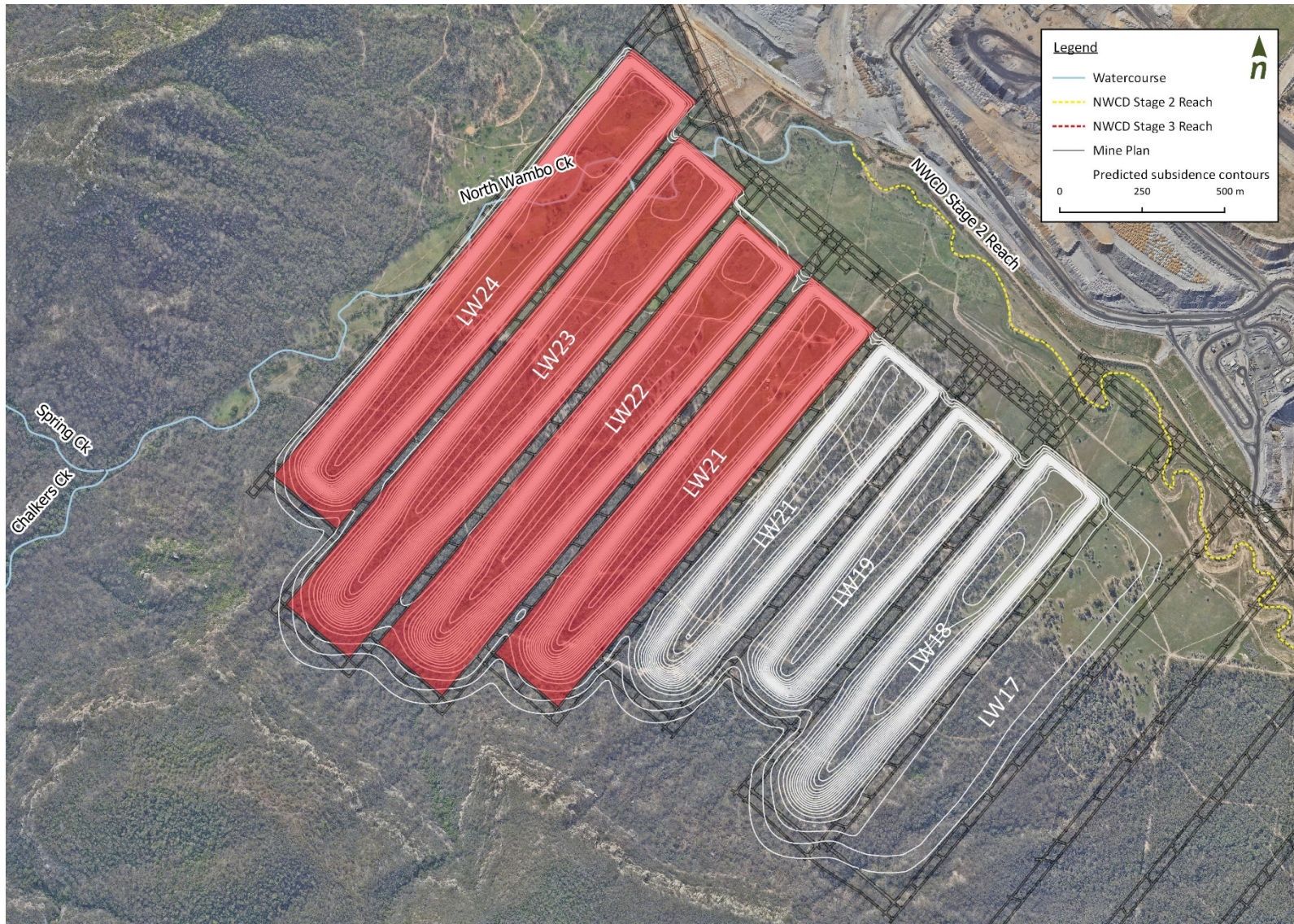
Figure 3-1. Predicted subsidence contours for South Bates Extension underground mine LW21 to LW24, including LW17 to LW20 (MSEC, 2020)
