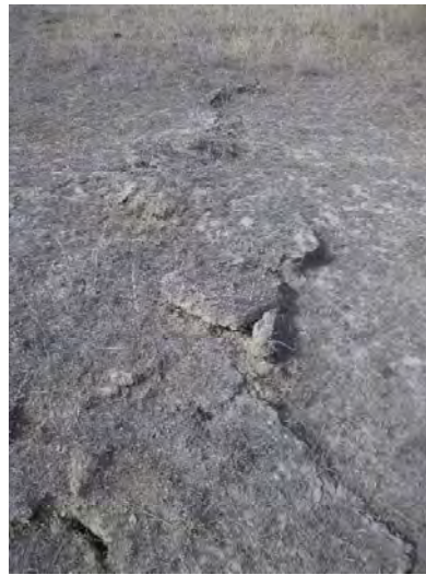
Fig. 4.5 Compression heaving above north-eastern end of WYLW17
