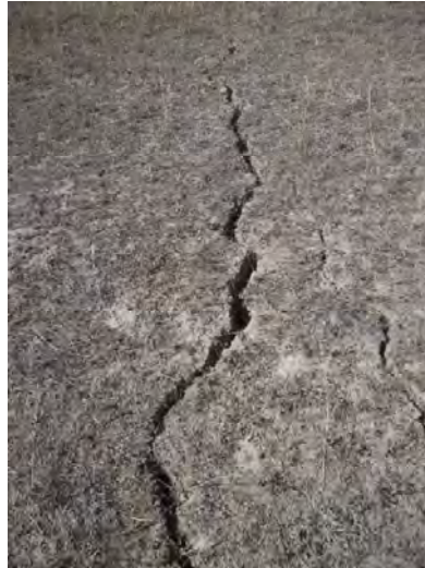
Fig. 4.4 Surface cracking above north-eastern end of WYLW17
