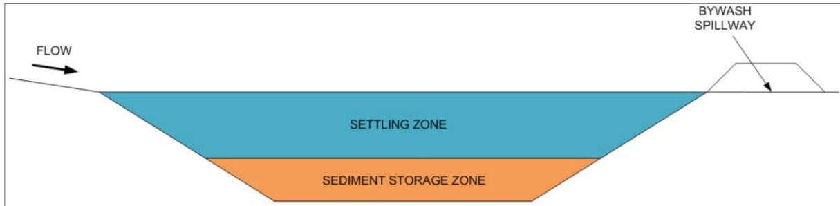
Figure 9: Settling and Storage Zones
