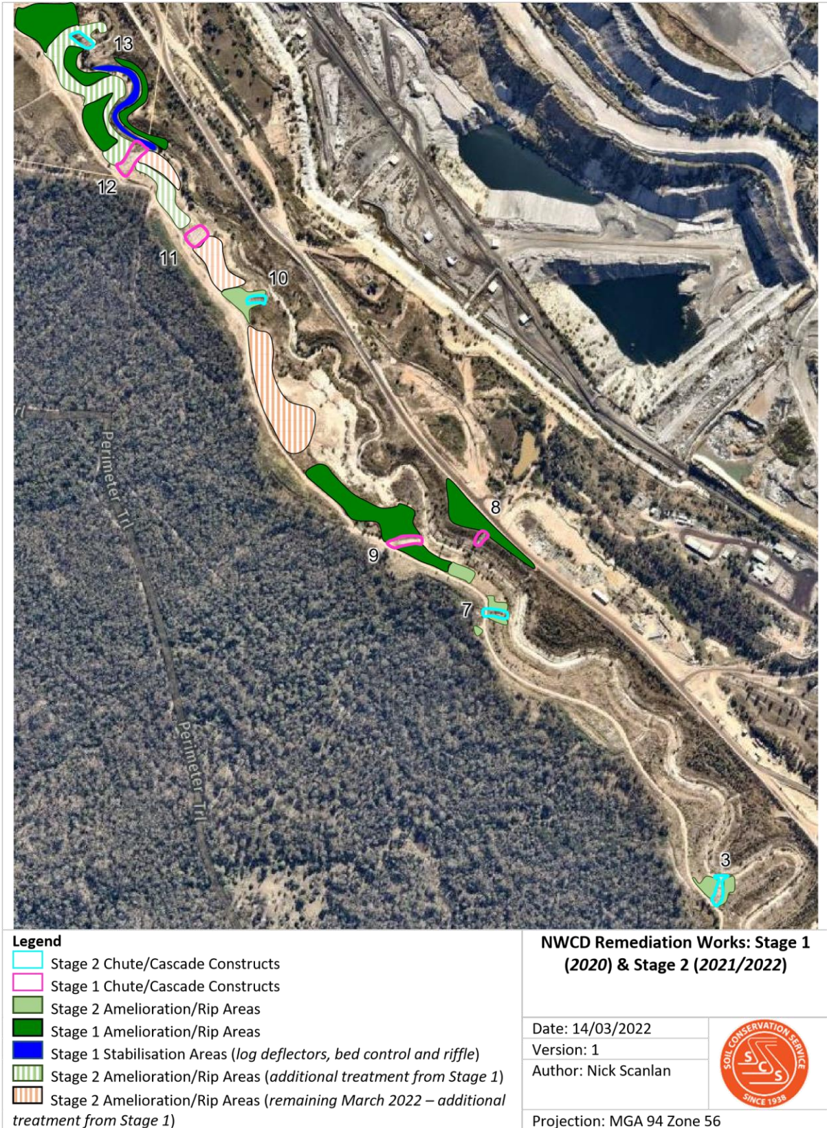
Figure 7: North Wambo Creek Remediation Works
