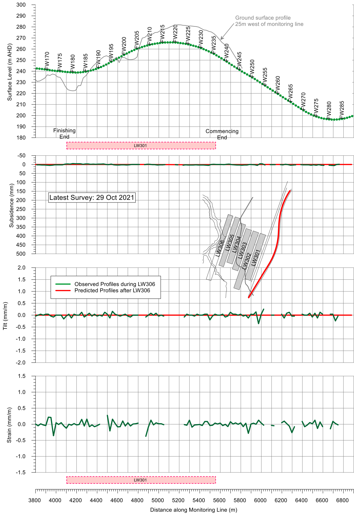
Fig. 2.1 Observed Incremental Subsidence Movements
