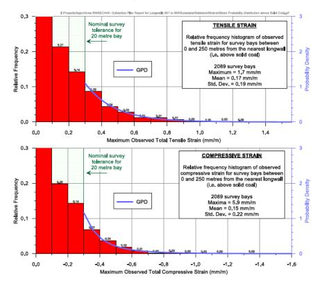
Figure 1 Distributions of the Measured Maximum Tensile and Compressive Strains during the Extraction of Previous Longwalls in the Southern Coalfield Above Solid Coal
