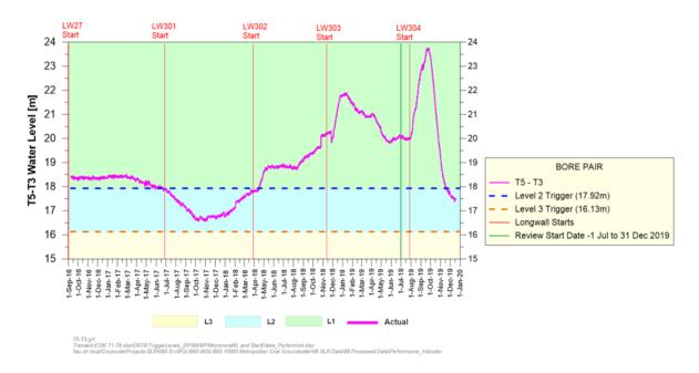
Chart 70 Hydraulic Gradient Measured from Bore T5 to Bore T3
