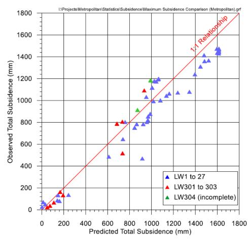
Chart 1 Comparison Between the Maximum Observed and Maximum Predicted Total Conventional Subsidence for Longwalls 3 to 27, Longwalls 301 to 303 and Partial Extraction of Longwall 304 at Metropolitan Colliery
