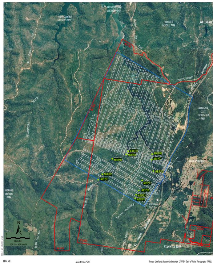
Mining Lease Boundary Railway Project Underground Mining Area Longwalls 20-27 and 301-317 Existing Underground Access Drive (Main Drift)
