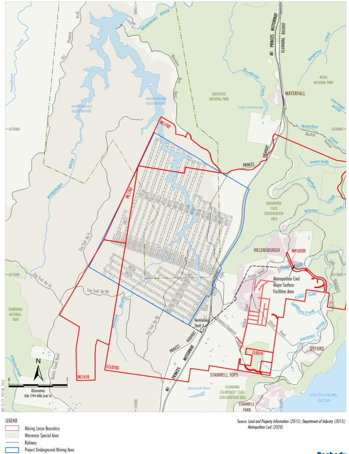
Project Underground Mining Area Longwalls 20-27 and 301-317 Woronora Notification Area Existing Underground Access Drive (Main Drift)
