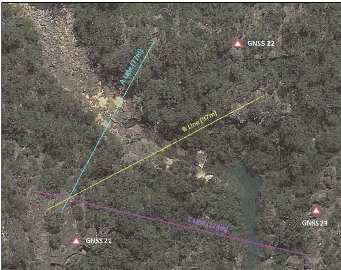
Figure 4.14 High precision survey lines across Eastern Tributary
