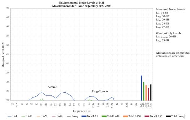
Figure 7: Environmental Noise Levels, N21 - Wambo South
