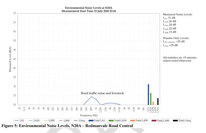
A low-level engine continuum from WCM was audible during the measurement, which generated the measured siteonly  $L_{Aeq}$  and  $L_{A1,1minute}$  of less than 25 dB.
