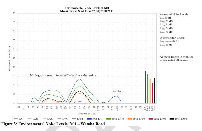
A mining continuum and track noise from WCM were audible throughout the measurement, generating a site-only  $L_{Aeq}$  of 31 dB. Track noise was responsible for the measured site-only  $L_{A1,1minute}$  of 37 dB.
