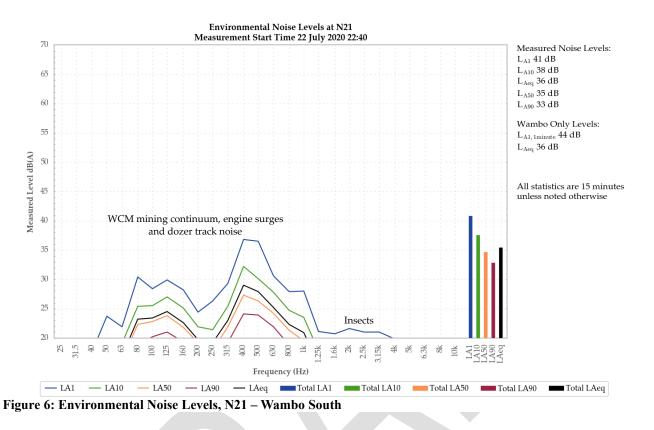
A mining continuum, engine surges and track noise from WCM were audible throughout the measurement, which generated a site-only  $L_{Aeq,15minute}$  of 36 dB. Track noise generated the site-only  $L_{A1,1minute}$  of 44 dB.
