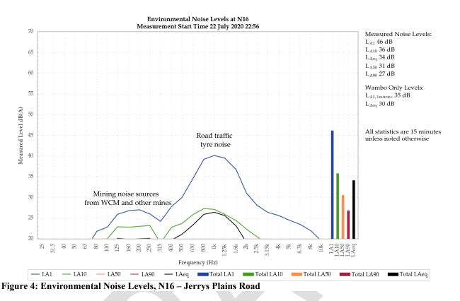
A mining continuum from WCM was audible throughout the measurement, which generated the site-only  $L_{Aeq}$  of 30 dB. Surges in the continuum generated the site-only  $L_{A1,1minute}$  of 35 dB. Engine surges were also noted.
