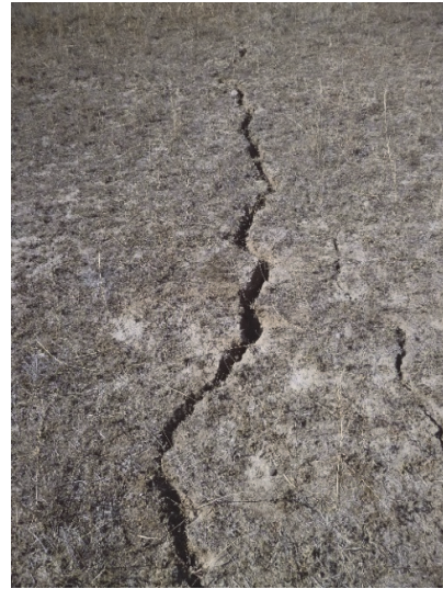
Fig. 4.4 Surface cracking above north-eastern end of WYLLW17
