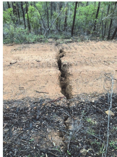
Fig. 4.11 Surface cracking along an access track above WYLW18 and WYLW19 (Source: WCPL)
