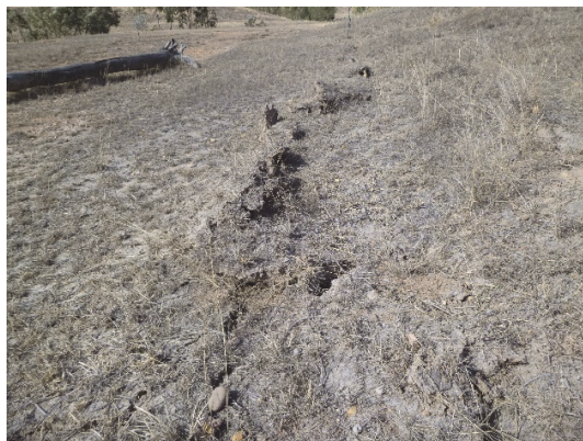
Fig. 4.5 Compression heaving above north-eastern end of WYLLW17
