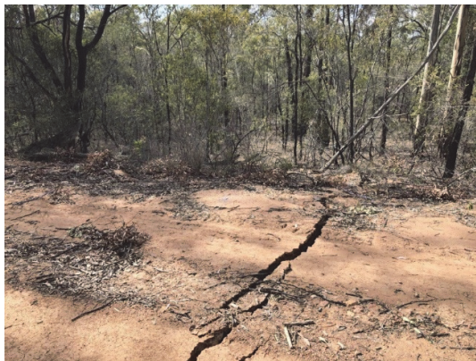
Fig. 4.11 Surface cracking along an access track above WYLW18 and WYLW19 (Source: WCPL)
