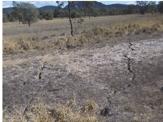
Fig. 4.7 Surface cracking above the middle of WYLW17
