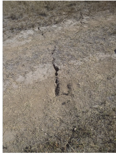
Fig. 4.6 Surface cracking along the access tracks above WYLW17
