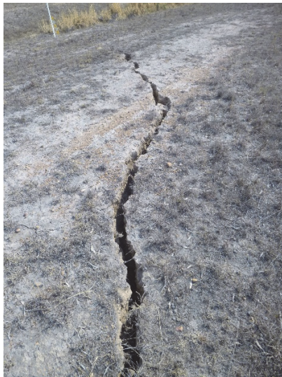
Fig. 4.7 Surface cracking above the middle of WYLW17
