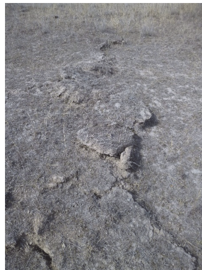
Fig. 4.5 Compression heaving above north-eastern end of WYLLW17
