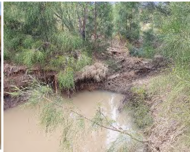
Head cut incision of channel bed in response to subsidence between LW16 and LW17
