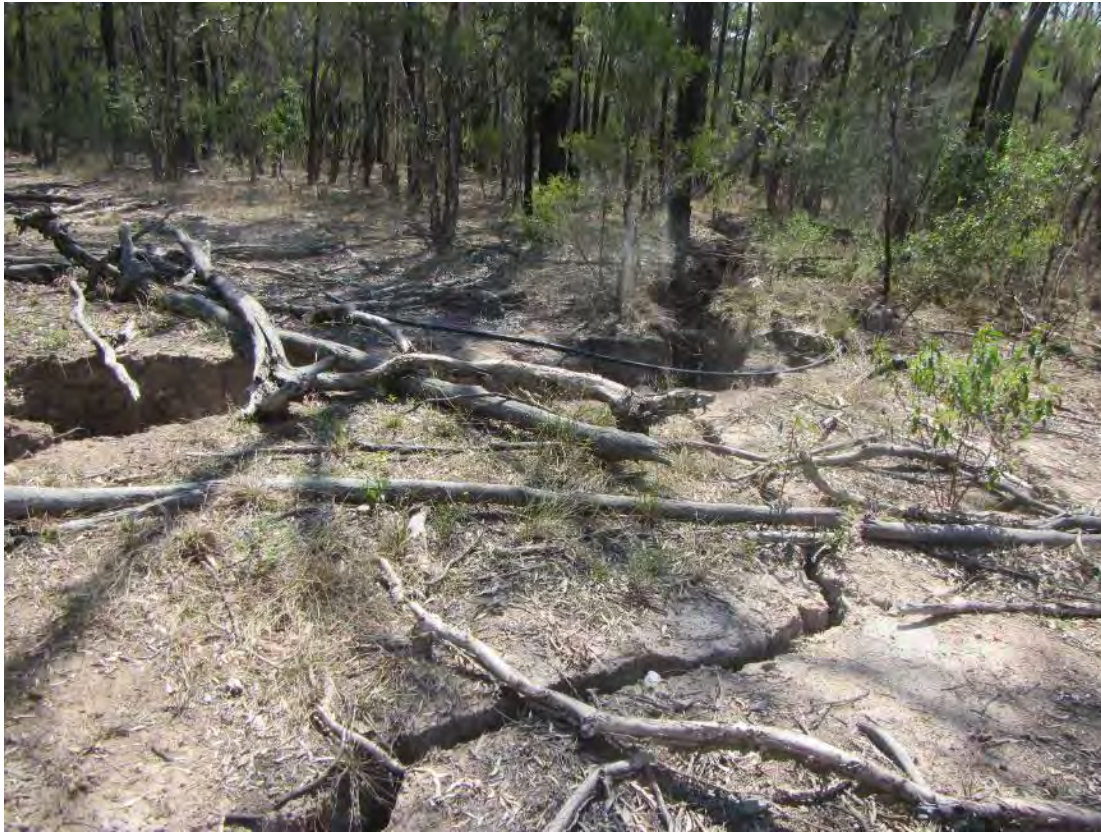
Figure 3-7. Large crack development example over LW11-16 in woodland east of NWCD
