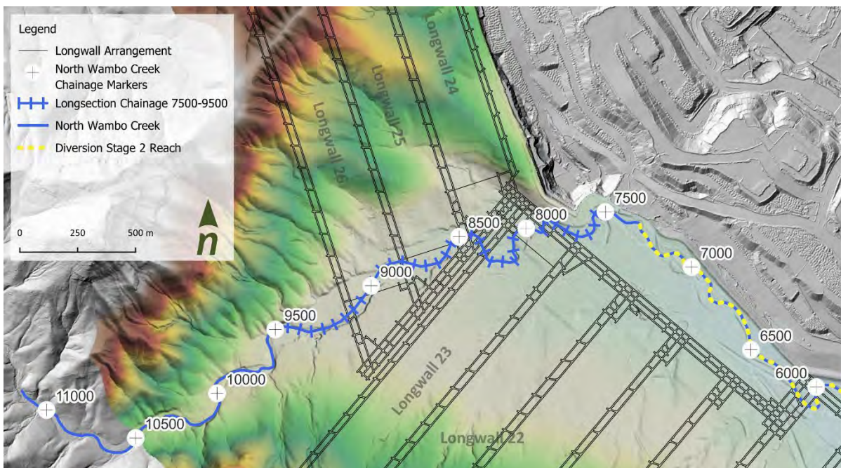
Figure 3-10. Predicted post subsidence surface over LW23, LW24 and LW25. Note the extents of macro channel and orientation of the channel in relation to the LW23, LW24-5 panel alignment.
