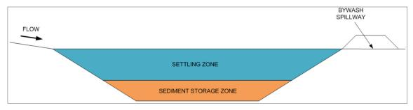
Figure 5: Settling and Storage Zones
