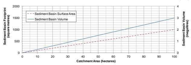
NB: An assumed basin depth of 3 metres and a target particle size of 500 micrometres has been used to derive the footprint area.
