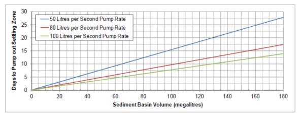
Figure 7: Indicative Pump Out Time Frames
