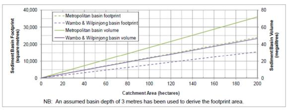
Figure 6: Indicative Sediment Dam Capacity
