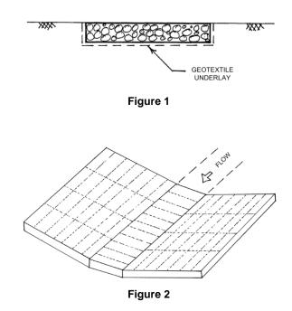
On dispersive soils it may be necessary to fill voids in the mattresses with soil or vegetation to help reduce erosion under the structure. Where rock mattresses are used for spillway construction, an additional layer of concrete shall fill the voids to reduce seepage through the mattress.
