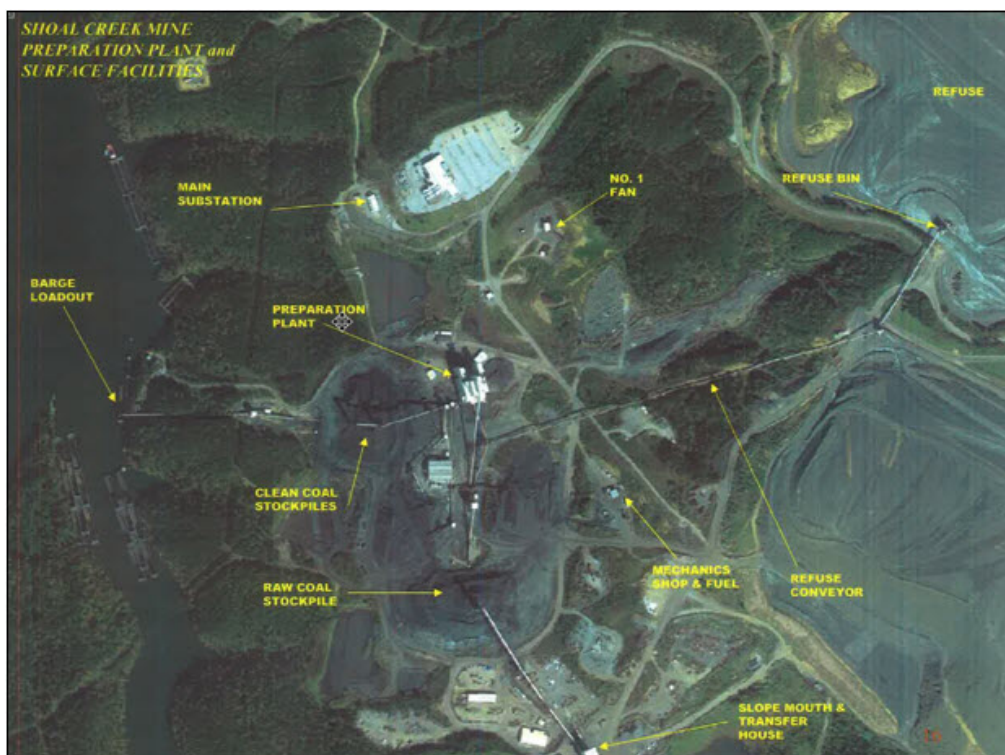
Figure 14-2. Preparation Plan & Surface Facilities
