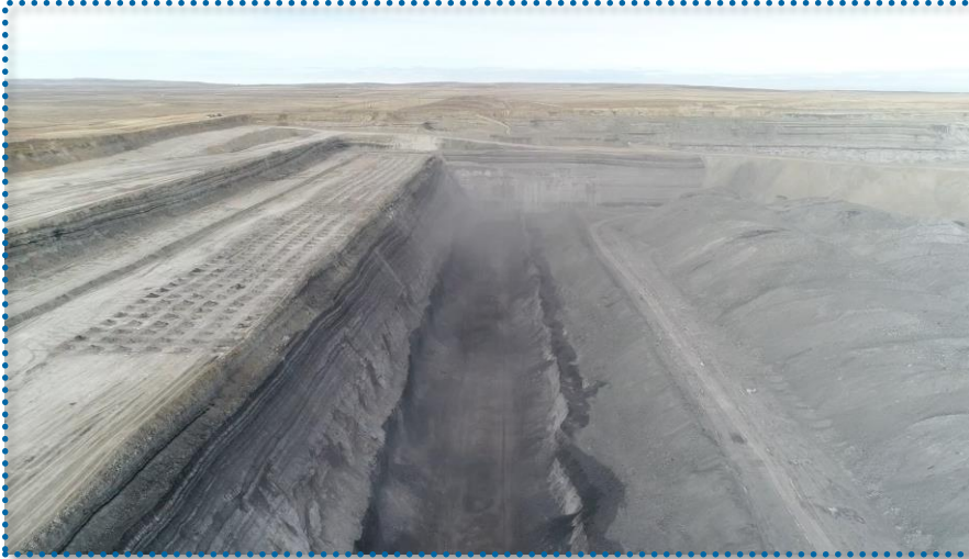
NARM cast blast, maximizing lowest-cost method of overburden removal
