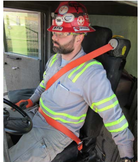
A Schroth auto-retracting, three-point seatbelt system in a CAT 785 truck.
