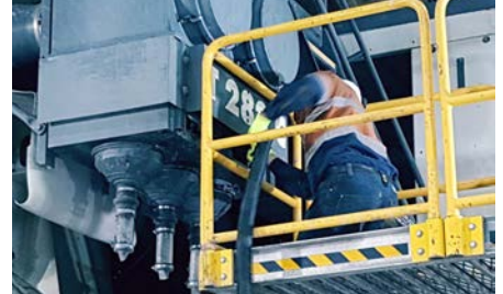
Cleaning with an industrial vacuum allows the task to be carried out with minimal exposure to dust.
