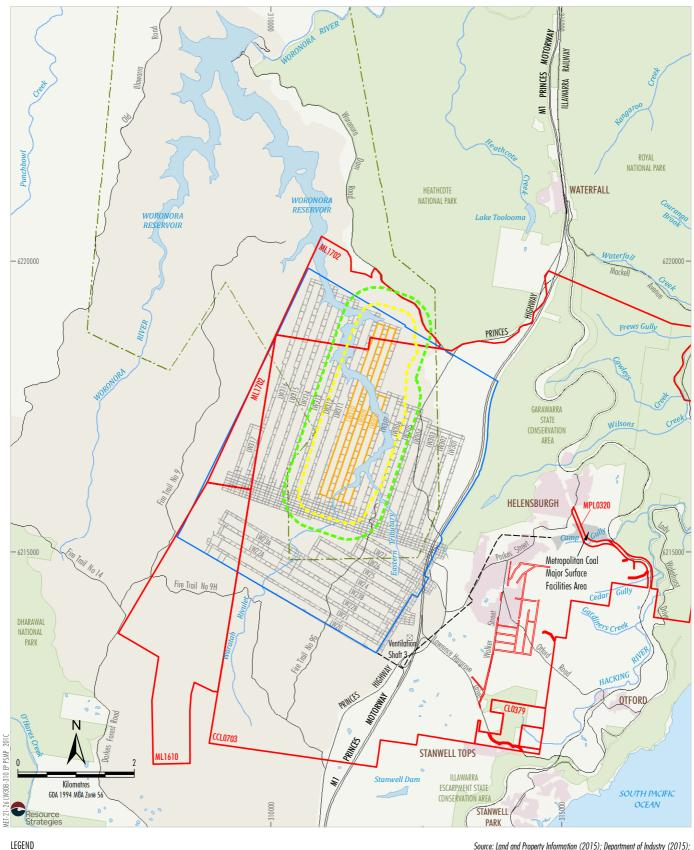
Mining Lease Boundary Woronora Special Area Project Underground Mining Area Longwalls 20-27 and 301-317 Longwalls 308-310 Secondary Extraction Longwalls 308-310 35° Angle of Draw and/or Predicted 20 mm Subsidence Contour 600 m from Longwalls 308-310 Secondary Extraction Woronora Notification Area Existing Underground Access Drive (Main Drift) Source: Land and Property Information (2015); Department of Industry (2015); Metropolitan Coal (2021); MSEC (2021)
