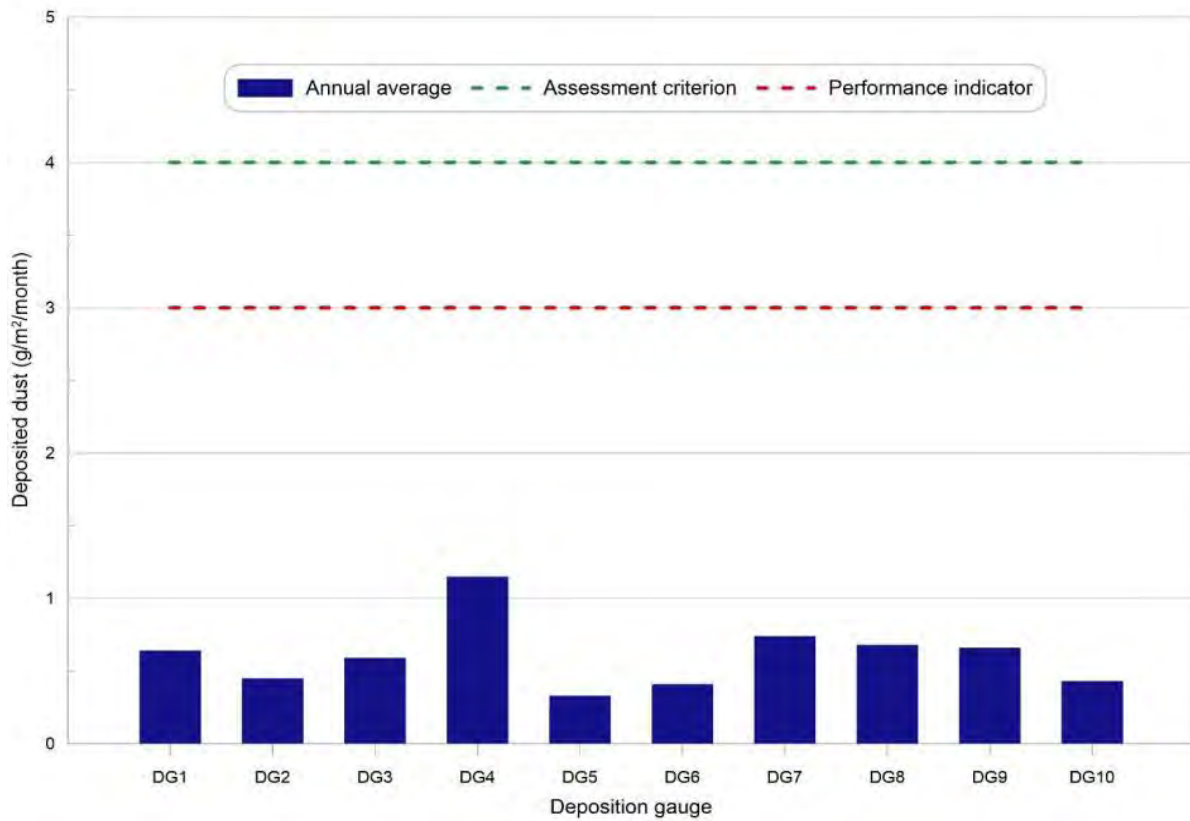
Chart 88 Annual Average Dust Deposition Rates Measured at Dust Gauges (DG1 to DG10)
