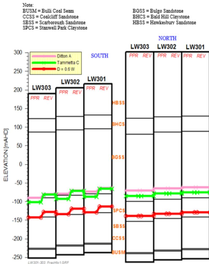
**Figure 6-5: Fracture zone height predictions using Ditton & Tammetta models**
