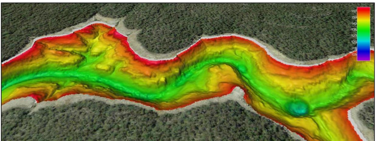
**Figure 6-10: Bathymetric survey results showing 3D image of reservoir floor for Waratah Rivulet.** Coloured levels are noted in mAHD. (Source: Ramsay et al., 2014)
