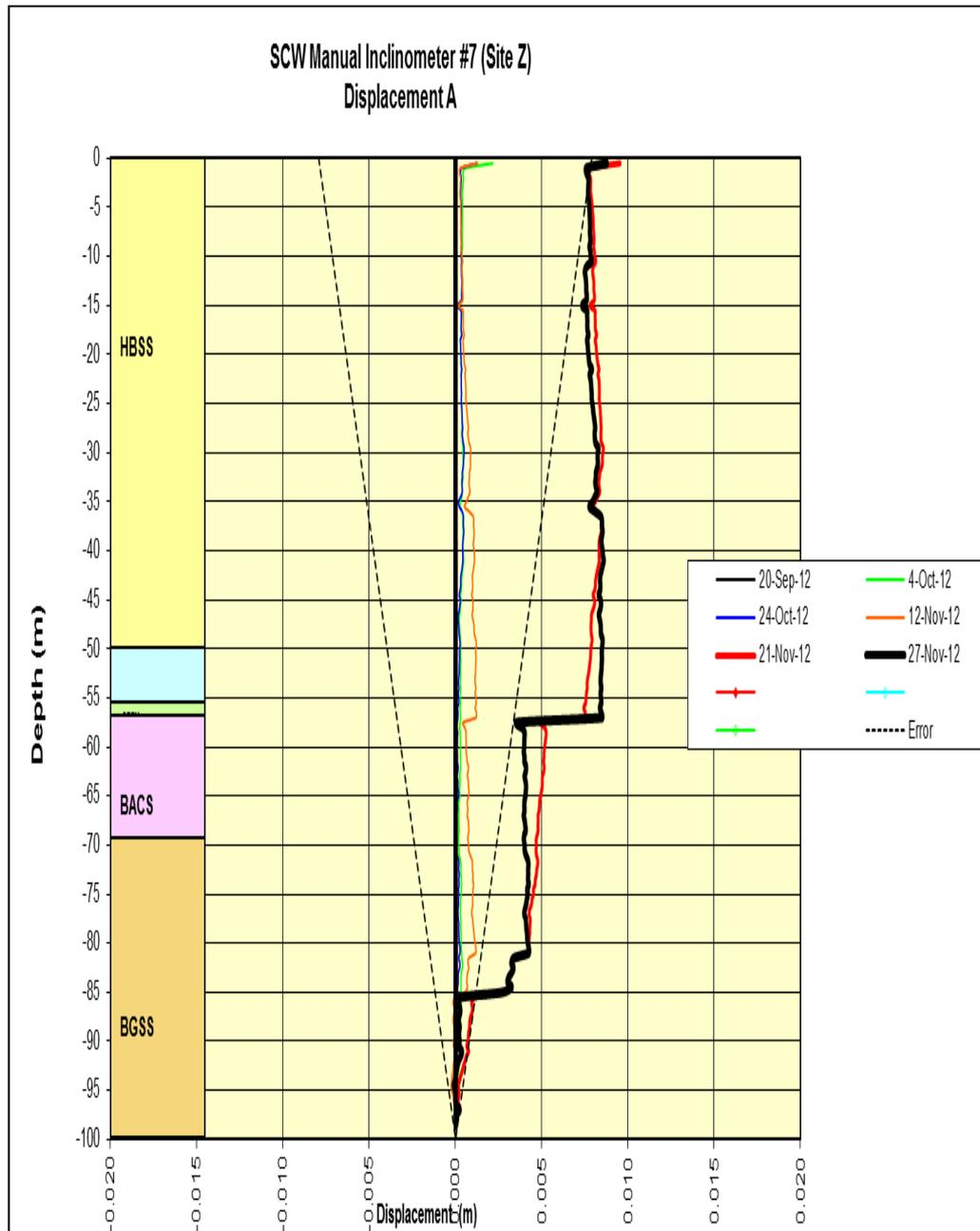
**Figure 6-6: Bedding plane shear detected above Dendrobium Mine, near Sandy Creek Waterfall, detected using borehole inclinometer. (source: Walsh et al., 2014)**
