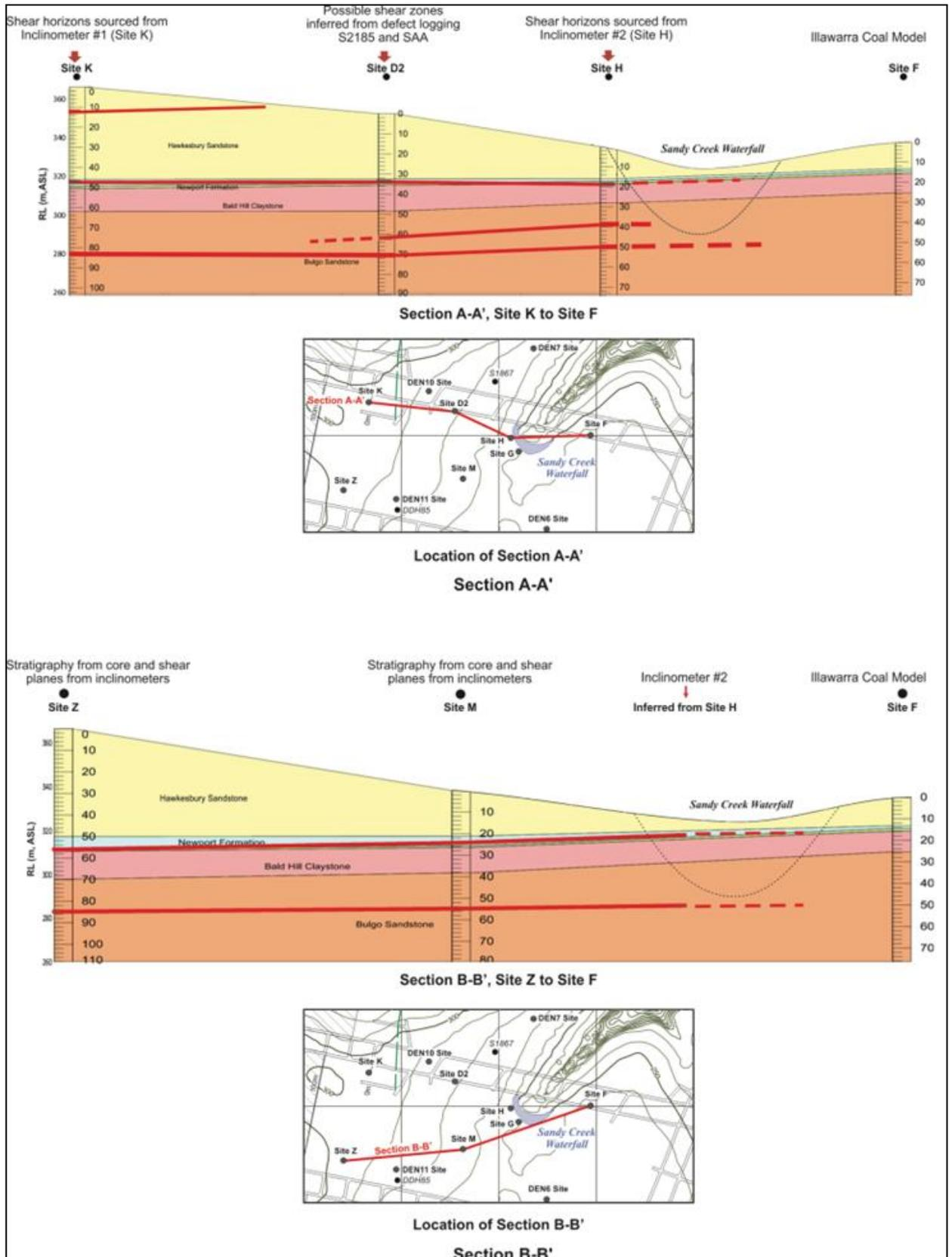
Figure 6-7: Correlation of near-surface shear movements relative to strata units - Dendrobium Mine, near Sandy Creek Waterfall. (source: Walsh et al., 2014)
