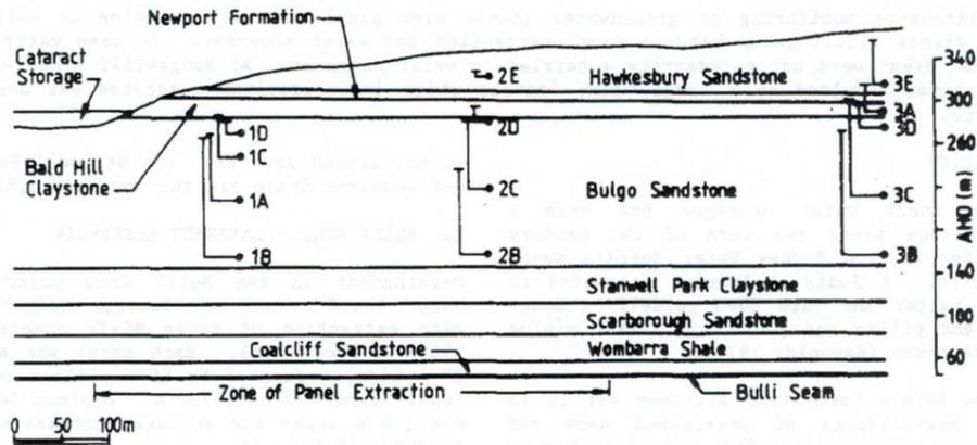
Figure 4-1: Stratigraphic section and piezometer locations (From Whitfield 1988).
