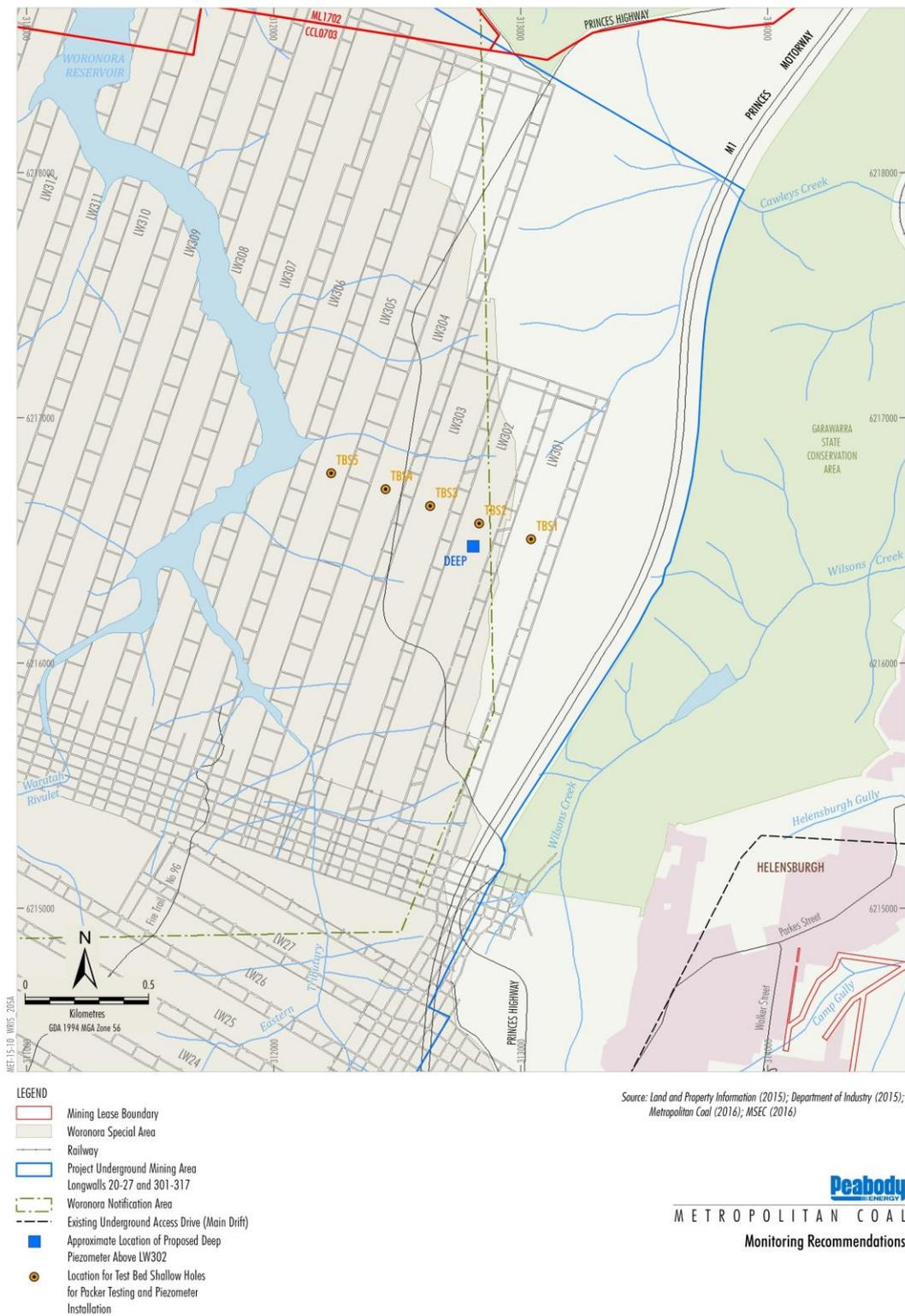
**Figure 5-1: Proposed locations for test bed boreholes for packer testing, VWP and standard piezometer installation TBS1 to TBS5 (TBS4 and TBS5 depending on access) and approximate location of proposed deep piezometer to goaf above LW302.**
