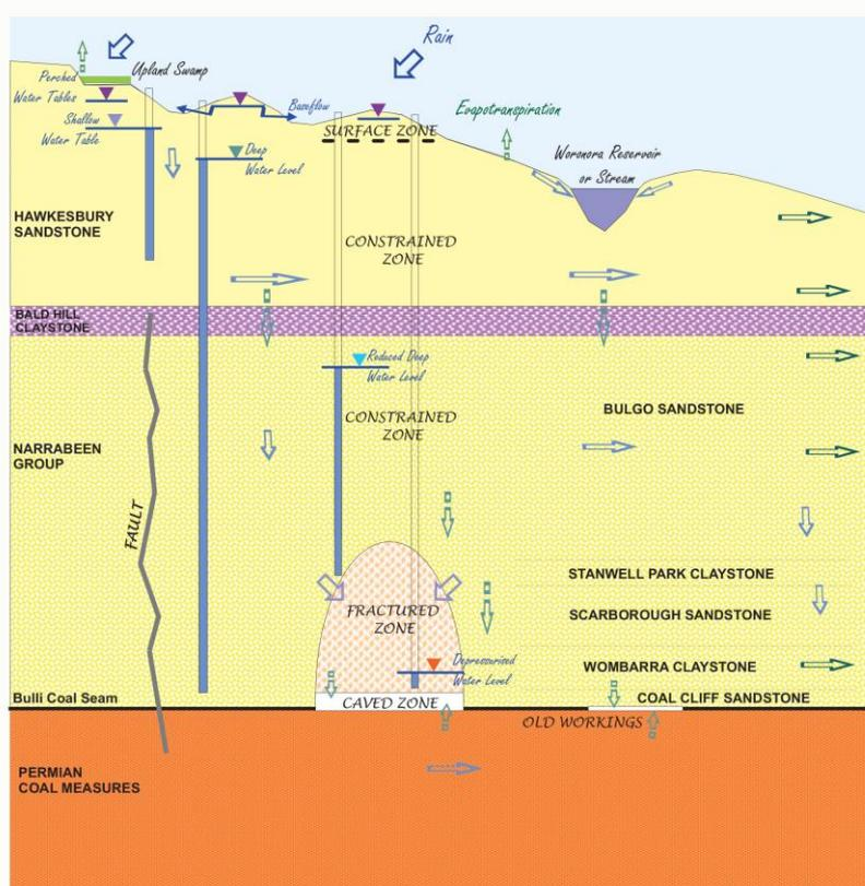
**Figure 3-1: Conceptual groundwater system for Metropolitan Coal mining conditions (Not to scale)**
