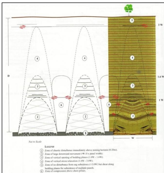
**Figure 6-4: Conceptual model of overburden caving behaviour above a longwall panel**
