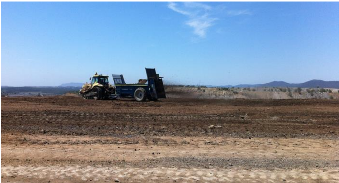
Plate 1 – Biosolid Application on Re-profiled Waste Rock Emplacement
