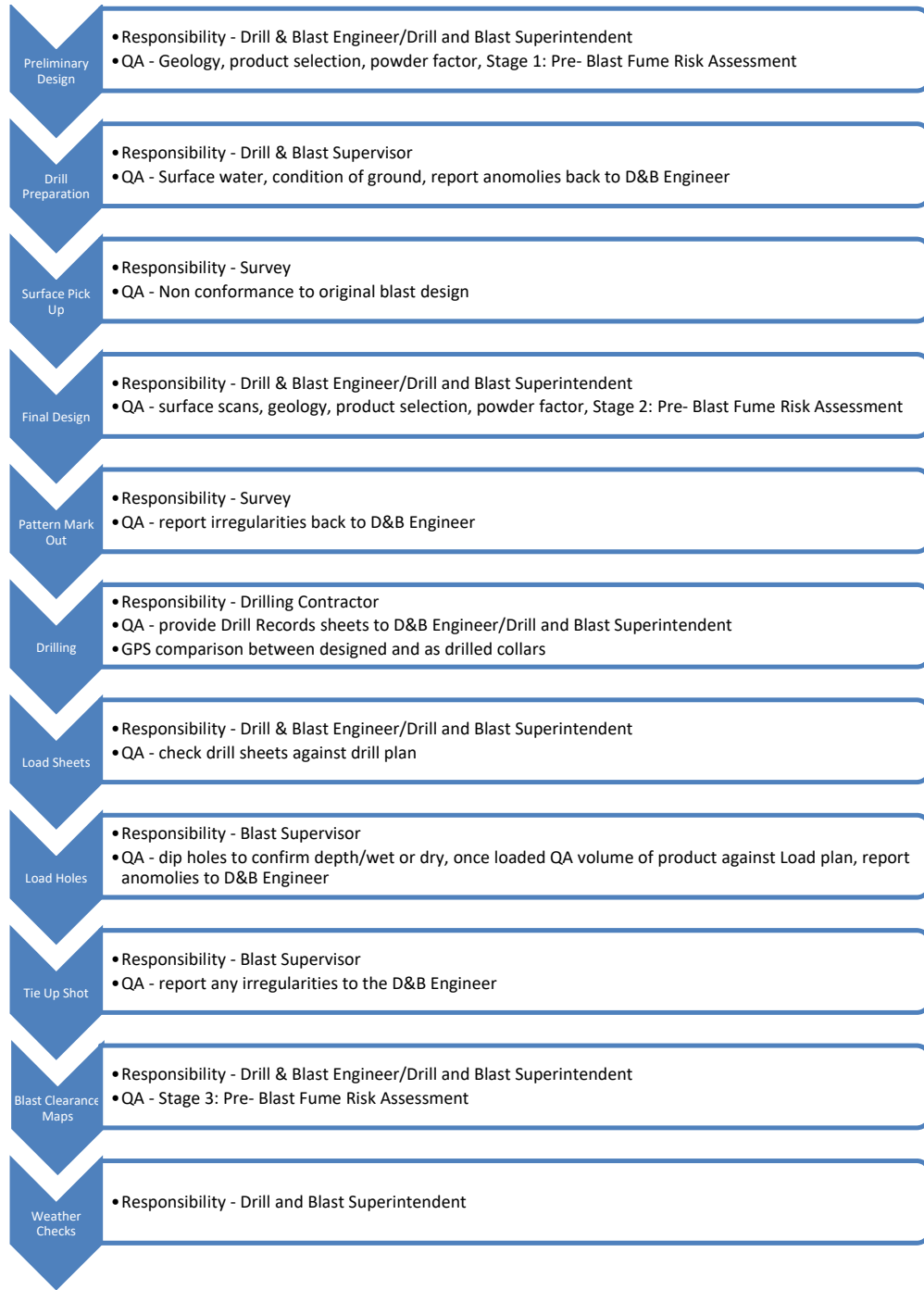
Figure 3: Blast Process Flowchart
