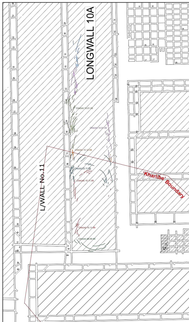
Figure 6: Location of cracks observed over Longwall 10A
