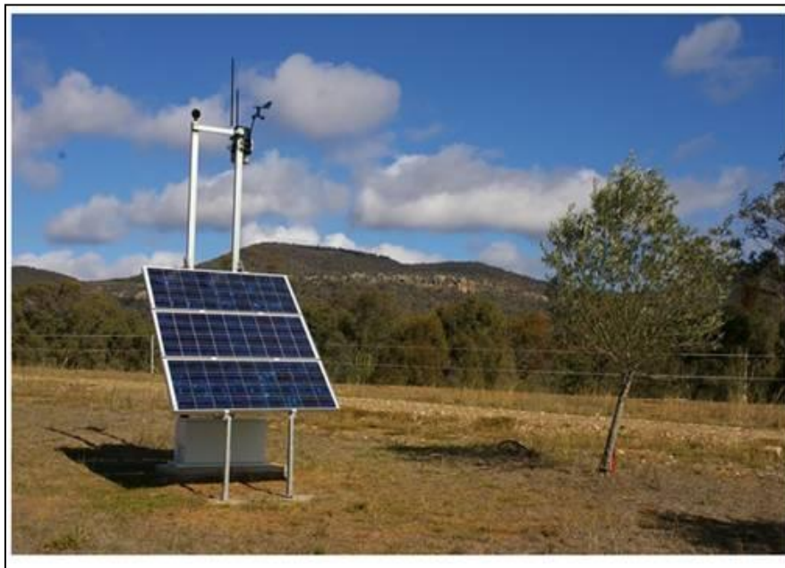
Figure 6: Real Time Noise Monitoring Unit at N20
