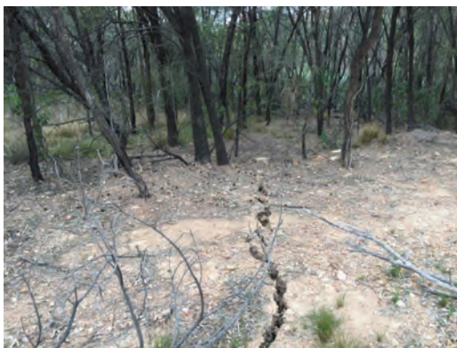
Fig. 4.7 Cracking along the fire trails above WYLW12 (Source: WCPL)
