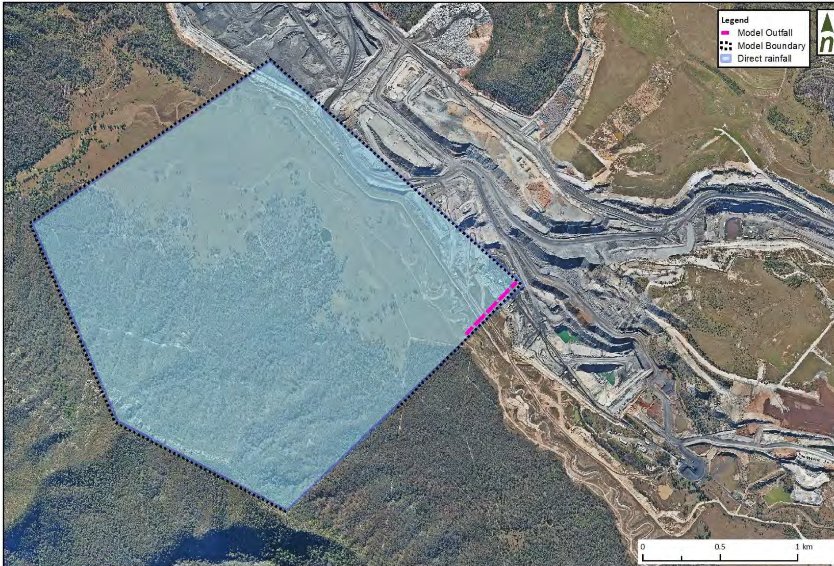
Figure C-0-2. 2D hydrodynamic 0.1% AEP model set up (existing conditions)
