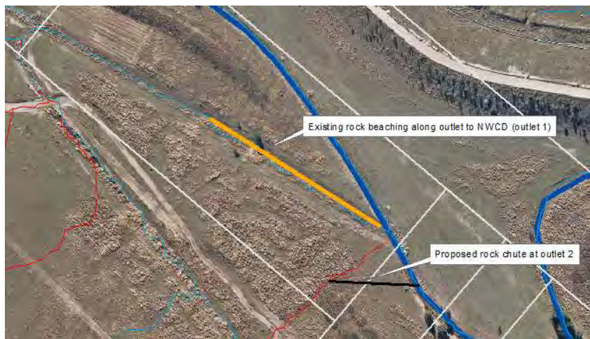
Figure D-0- 2. Plan view showing approximate location of existing rock beaching at outlet 1
